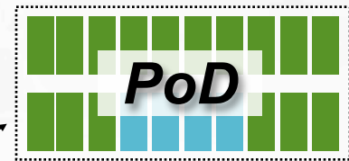
20 cabinet PoD with 16 server cabinets and 4 switch cabinets
